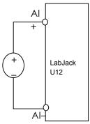
Fig.3. The voltage signals' differential connection
