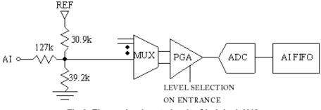
Fig.2. The analog input circuit of LabJack U12
