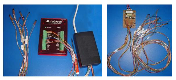
Fig.9. Data acquisition card and the LM 35 sensors
