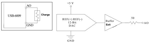
Fig. 6. Charge connection
